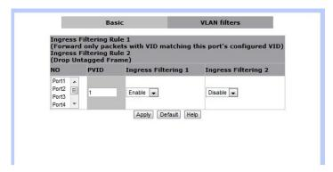
VLAN filter function is for setting the filtering rules for all ports (Port1 ~ Port24, Mod1 and Mod2).
