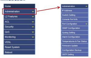
"Administration" section is for users to manage the VDSL2 IP DSLAM, including the IP address, switch settings, etc. It includes the following detail functions.
