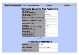
"System Configuration" allows users setting up the details of STP function. In addition, the information of the root node of the STP will be displayed in this page.
