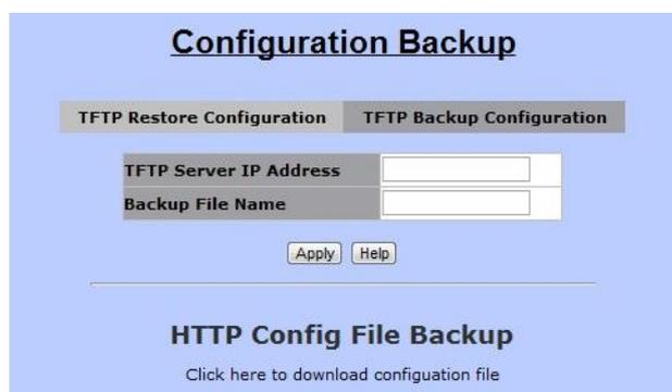
This area allows users to download the current configuration through TFTP or HTTP.
