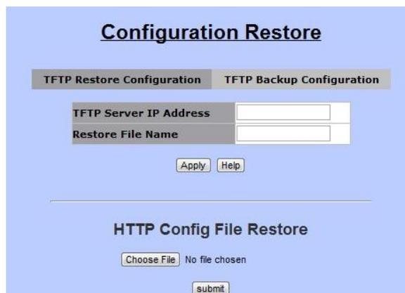
This section is for load the settings from a configuration file. Users are able to upload the settings by TFTP or HTTP.
