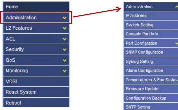
“Administration” section is for users to manage the MINI IP DSLAM, including the IP address, switch settings, etc. It includes the following detail functions.
