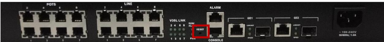
The reset button allows users to reboot the 8 Port Mini IP DSLAM or load the default settings.
