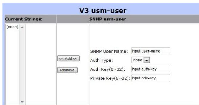
“SNMPv3 USM-User” section is for setting up the details of USM (User-based Security Model) security model. USM provides different types of security levels using various authentication and privacy protocols.
