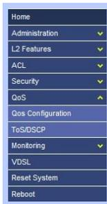
This switch provides quality of service (QoS) to prioritize the packet forwarding when traffic congestion happens. This switch supports two QoS functions: port-based (4-level output queue) and 802.1p (8-level priority to 4-level queue mapping). In addition, Strict and weight Round Robin (WRR) QoS modes are supported.
