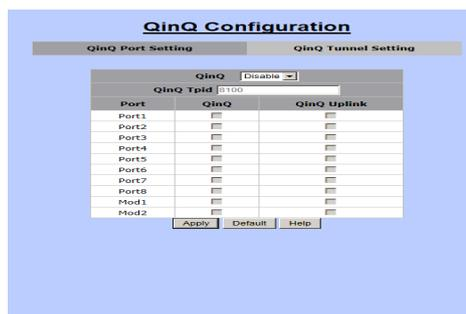
“Qinq Tunnel” is for service providers who carry traffic of multiple customers across their networks and are required to maintain VLAN and Layer 2 protocol configurations for each customer.
