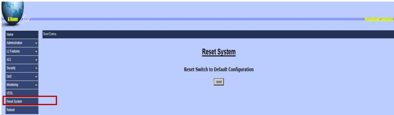
“Reset System” is for restoring all configurations back to the default factory configurations. All the settings will be changed back to the original state.
