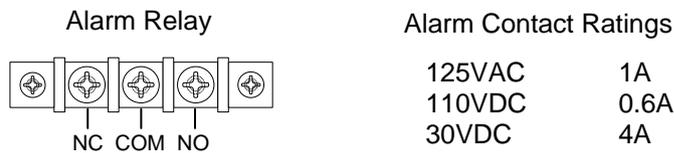
Figure 2-5 Alarm Relay Contacts
