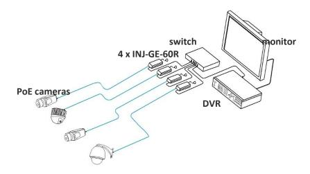
The INJ-GE-60R PoE Injector is used with various PD (powered devices) providing power in remote locations where no power lines or outlets are available. Examples of PD PoE powered devices are WiFi APs, IP Cameras, IP Phones, etc.
