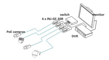
The INJ-GE-30R PoE Injector is used with various PD (powered devices) providing power in remote locations where no power lines or outlets are available. Examples of PD PoE powered devices are WiFi APs, IP Cameras, IP Phones, etc.
