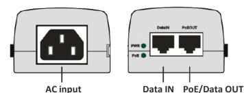
**PWR:** Power LED - a steady green light indicates that the PoE injector receives 100-240V AC power input
