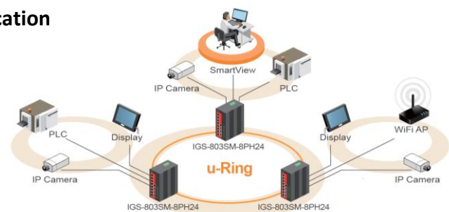
Figure 7. u-Ring Topology and Application
