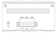
A removable terminal block provides both power and alarm connections. Power can be provided through the dual inputs from separate sources. One electrical relay can be wired into an alarm circuit. The relay is connected as Normally Closed (will open upon alarm condition).
