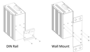
**IGS-401F/402F(S)** with DIN Rail bracket has a steel spring in the upper rail of the bracket. This spring is compressed for mounting and un-mounting by applying downward force.
