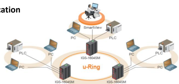
Figure 6. u-Ring Topology and Application
