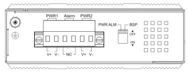
A removable terminal block provides both power and alarm connections. Power can be provided through the dual inputs from separate sources. One electrical relay can be wired into an alarm circuit. The relay is connected as Normally Closed (NC).
