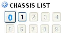
Use the "Chassis List" control to select the chassis in the cascade group. Using only one IP address and one single point of management, up to 10 chassis (ID 0~9) can be managed.
