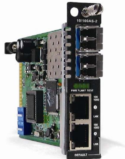
10/100AS-2 is a stand-alone manageable 4 port Fast Ethernet fiber switch, utilizing SFP for 100Base-FX fiber connection and two 10/100 Ethernet electrical ports.
