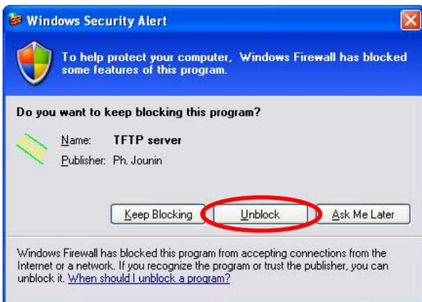
Start the TFTP server on the connected PC. In our example, we are using the free tftp32 TFTP server. If Windows® is running a firewall, a security alert will popup. Click the "Unblock" button to allow TFTP protocol from the TFTP Server application.
