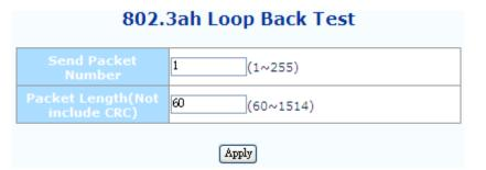
The loop back test is a non-intrusive test which uses OAM packets and will not affect normal transmissions. The number of OAM frames used (the number of times the loop back is done) is set by the **Send Packet Number**. The default is 1 packet.
