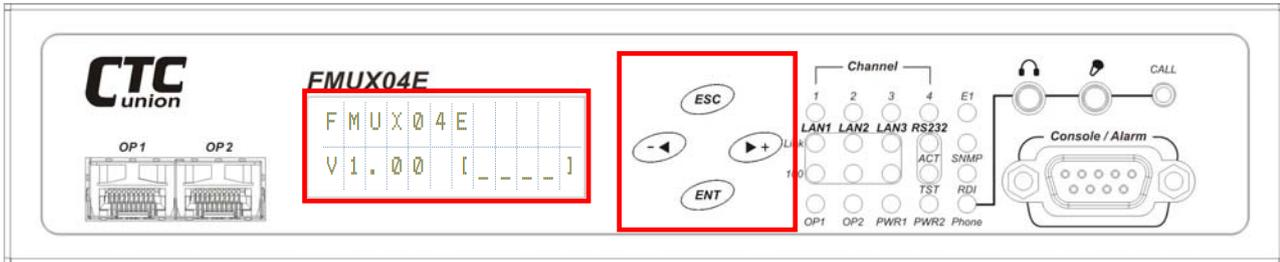
The 12 character by 2 line LCD is located plainly on the front panel. To its right are the 4 menu keys.
