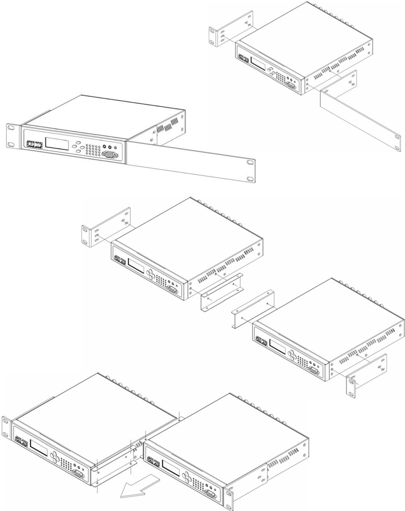
Figure 2-2. Single and tandem rack mounting of FMUX04E.
