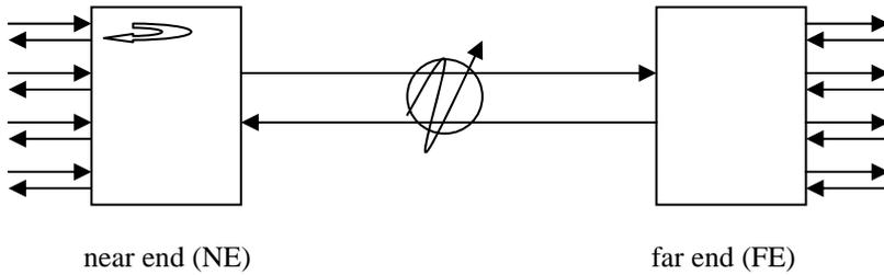
This local loop back will make the near end unit loop towards the copper side's channel.
