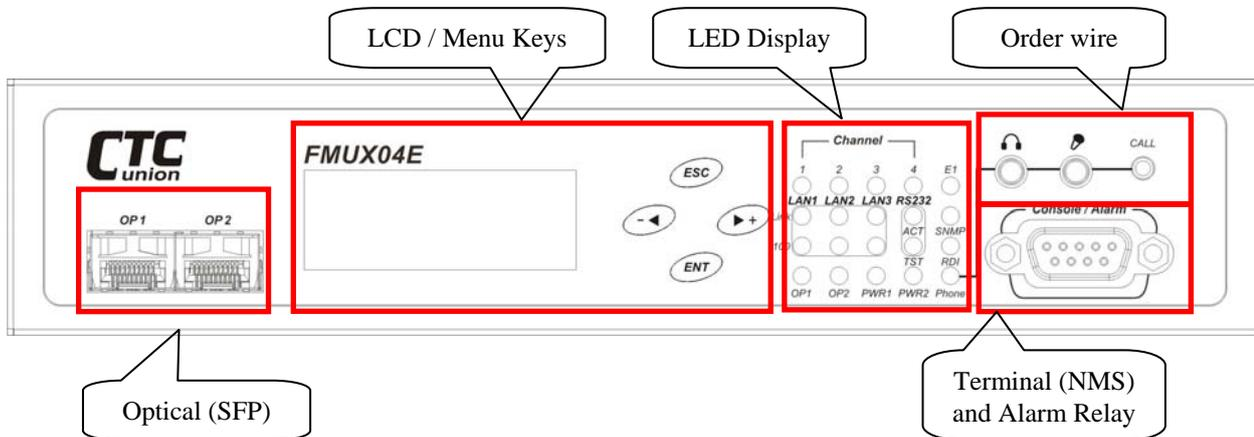
Figure 2-5 : Front Panel Controls and Indicators
