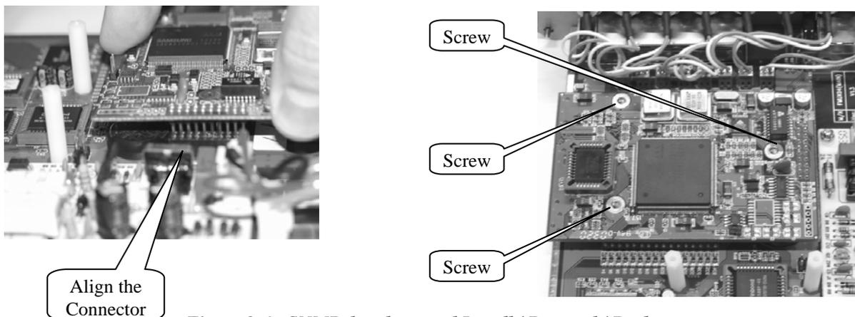
Figure 2-6 : SNMP daughter card Install / Removal / Replacement
