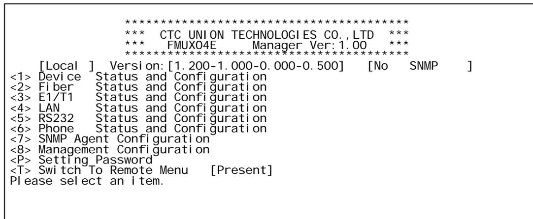
Just below the main header, we find the [Local] shown in brackets. This is the main menu for the local unit. The Version explanation for the example shown here is PCB h/w version 1.200, s/w version 1.000, CPLD version 0.000 (or none) and FPGA version 0.500.
