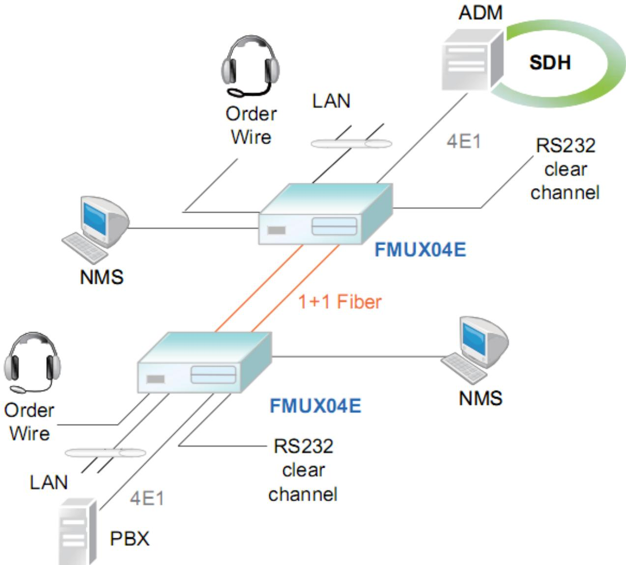
Figure 1-2 : Typical Point-to-Point Application of FMUX04E
