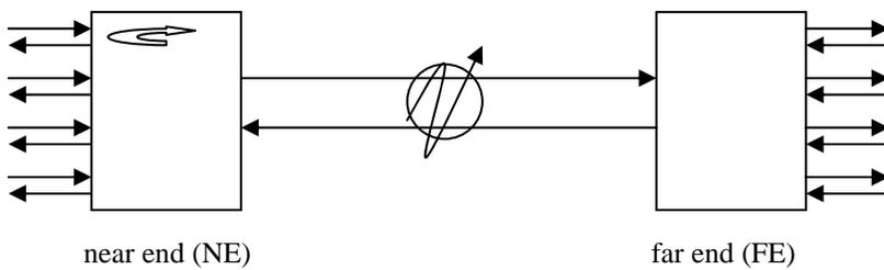
This remote loop back will loop the logical channel from the near end unit back to the far end unit via the fiber.
