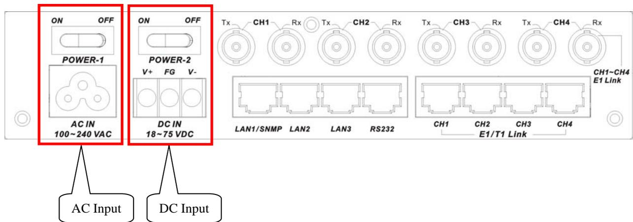
Figure 2-3 : Supply connections, AC+DC model shown
