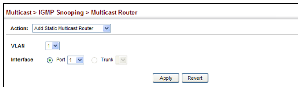
Figure 235: Configuring a Static Interface for a Multicast Router
