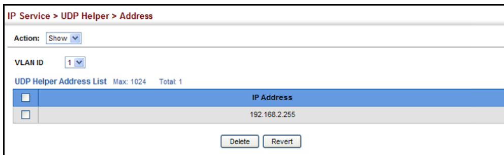
Figure 323: Showing the Target Server or Subnet for UDP Requests
