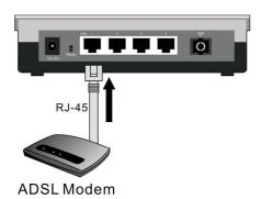
2. Connect the other end of the Ethernet cable to the **WAN** port of the Smart Router. (insert pic)
