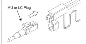
3.Push the Outer Shell to start cleaning the MU/LC connector end face. A "click" sound indicates end of cleaning process. Close the cover after use.
