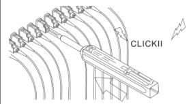
Be careful not to slant the RB-PEN125 while inserting into the adapter.
