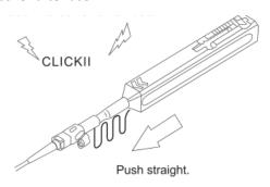
Be careful not to slant optical connector while inserting into the Guide Cap.
