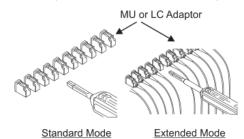
3. Push the Outer Shell to start cleaning the MU/LC connector end face. A "click" sound indicates end of cleaning process. Close the cover after use.
