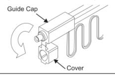
2.Insert MU/LC connector into the Guide Cap.
