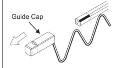
2.Insert tip of cleaner into MU/LC Adapter.
