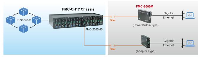
Figure 3: As Standalone Managed Converter
