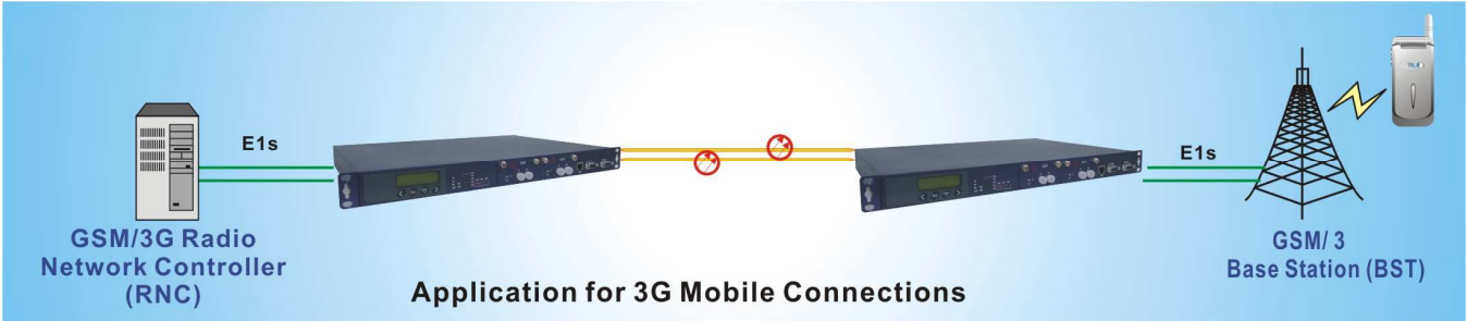
Figure 2-1 Terminal Multiplexer (TM) application
