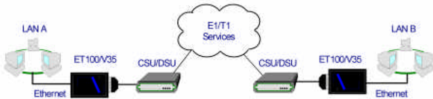
Typical application of ET100 LAN-WAN Bridge.
