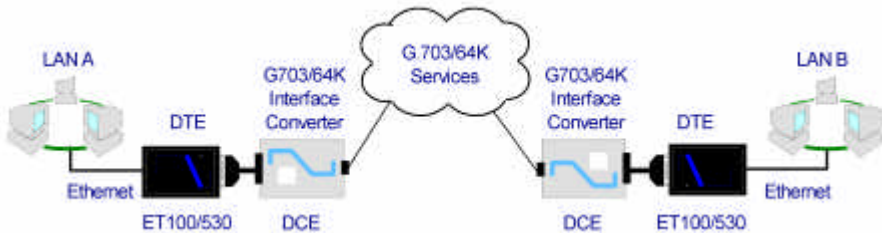
Figure 6: ET100 bridge over G.703 64K services.
